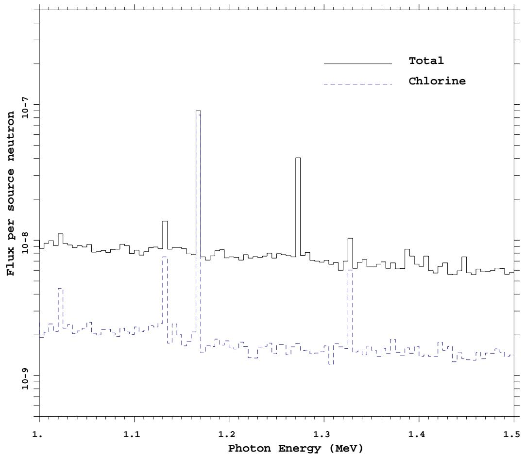
Figure 1. MCNP simulated photon spectra over the energy range  $E_{\gamma}=1.0-1.5$  MeV. The total photon spectra is indicated by the solid line and the contribution from thermal neutron capture reactions in Cl (13600 ppm) is given by the dashed line.
