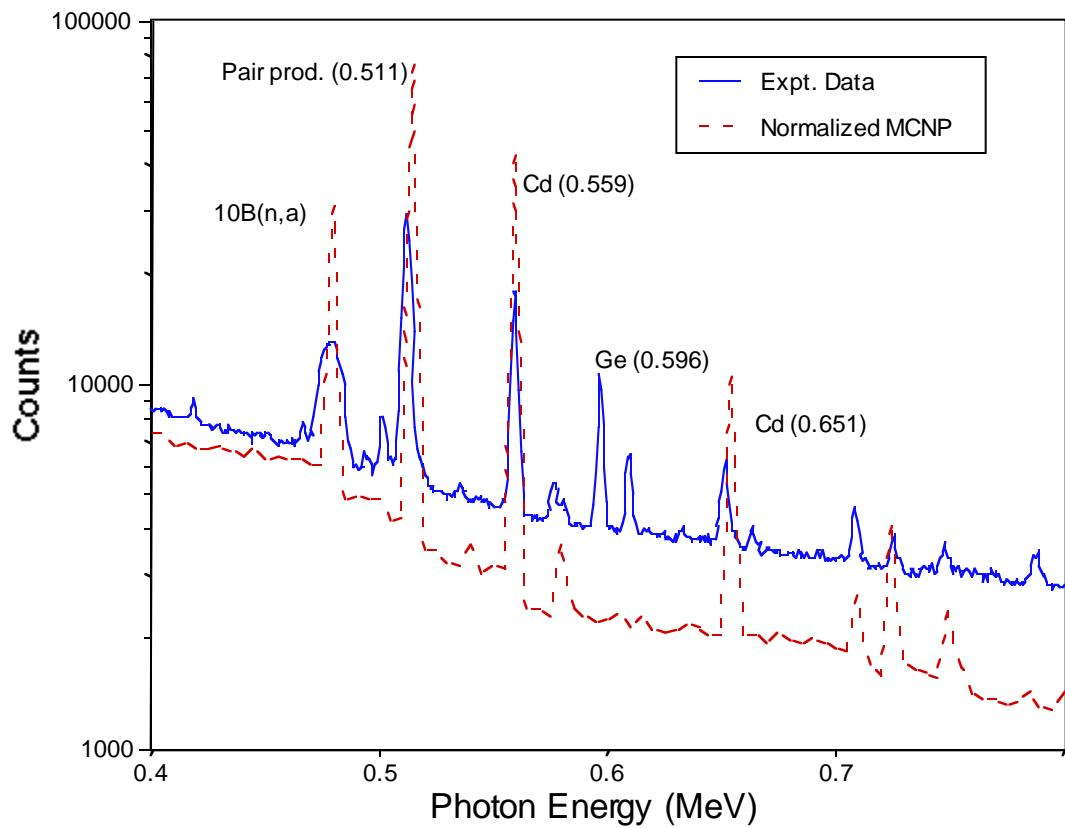
Figure 2. A comparison of experimental data (solid line) and normalized MCNP simulated photon spectra (dashed line) for Cd over the energy range  $E_{\gamma}$  = 0.4-0.8 MeV. The MCNP data is given in flux per source neutron and has been normalized to counts for comparison purposes.
