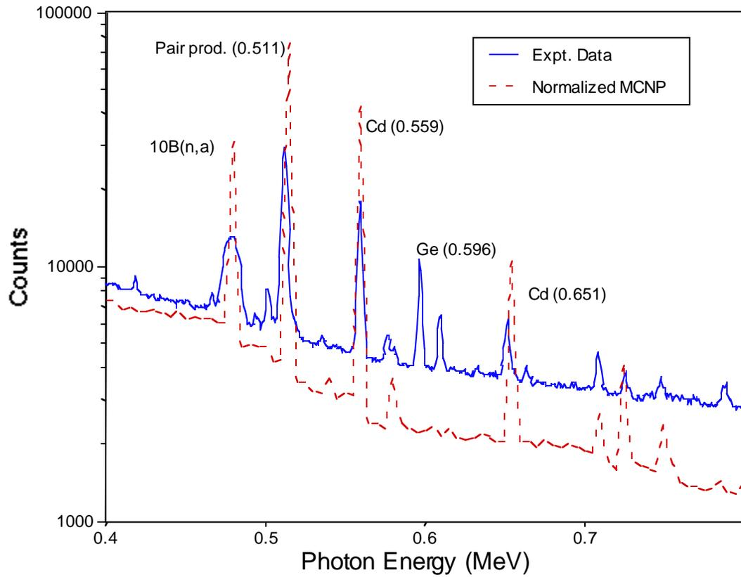
Figure 2. A comparison of experimental data (solid line) and normalized MCNP simulated photon spectra (dashed line) for Cd over the energy range  $E_\gamma = 0.4\text{-}0.8$  MeV. The MCNP data is given in flux per source neutron and has been normalized to counts for comparison purposes.
