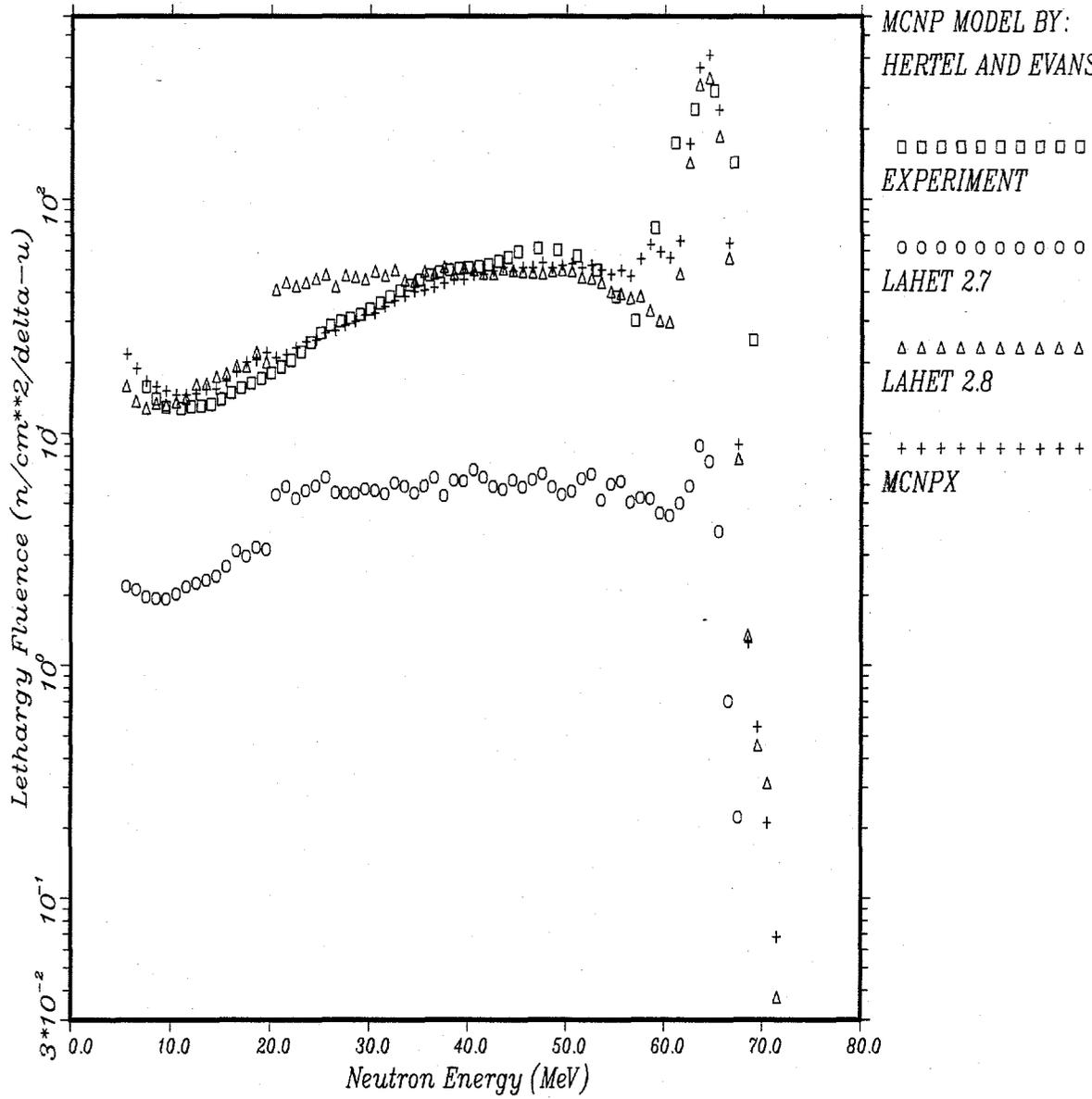
Fig. 2. Comparison of LAHET 2.7, LAHET 2.8 and MCNPX with experimental results in the JAERI experiment. The transmitted neutron fluence is measured and calculated immediately adjacent to the downstream side of the iron transmission target at a position 20 cm away from the beam centerline.
