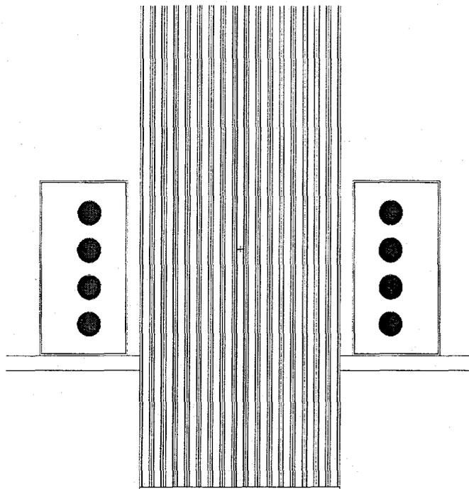
Fig. 3. MCNP model showing a slice through both heads of the detector, each with four  $^3\text{He}$  detector tubes, with the 17 x 17 fuel bundle centered between the heads.
