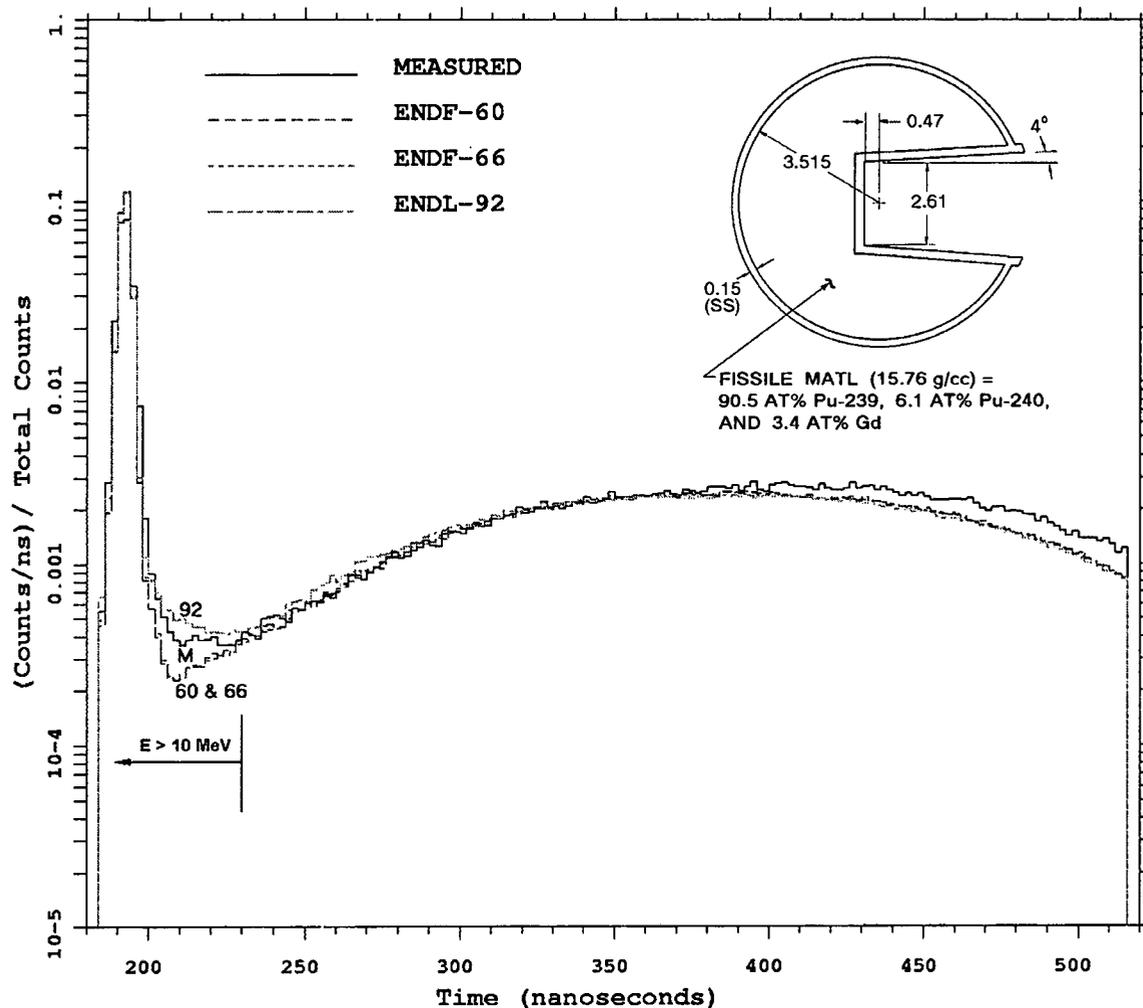
Fig.1. Results for the NE213-A neutron detector in the 120-deg beamline in combination with the 0.7 mfp Pu-239 pulsed sphere. Dimensions of sphere are in cm.
