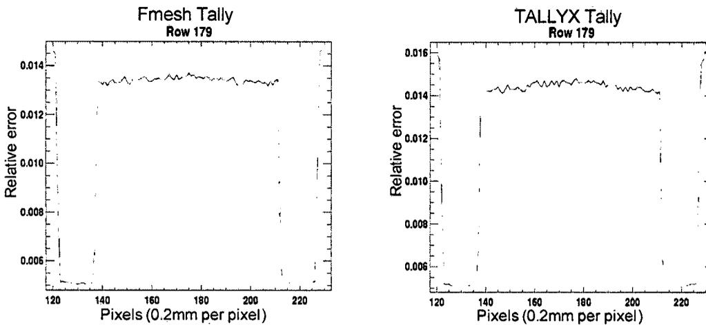
Figure 10- Line outs of the relative error for the fmesh and TALLYX tallies for cylinder 4.
