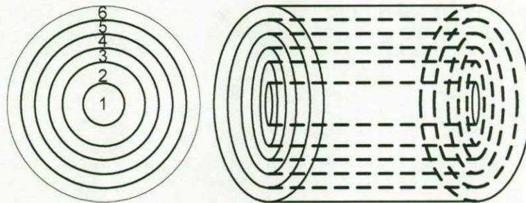
Figure 2 – Front and side views of the cylindrical target used for the cell tagging tally simulations.
