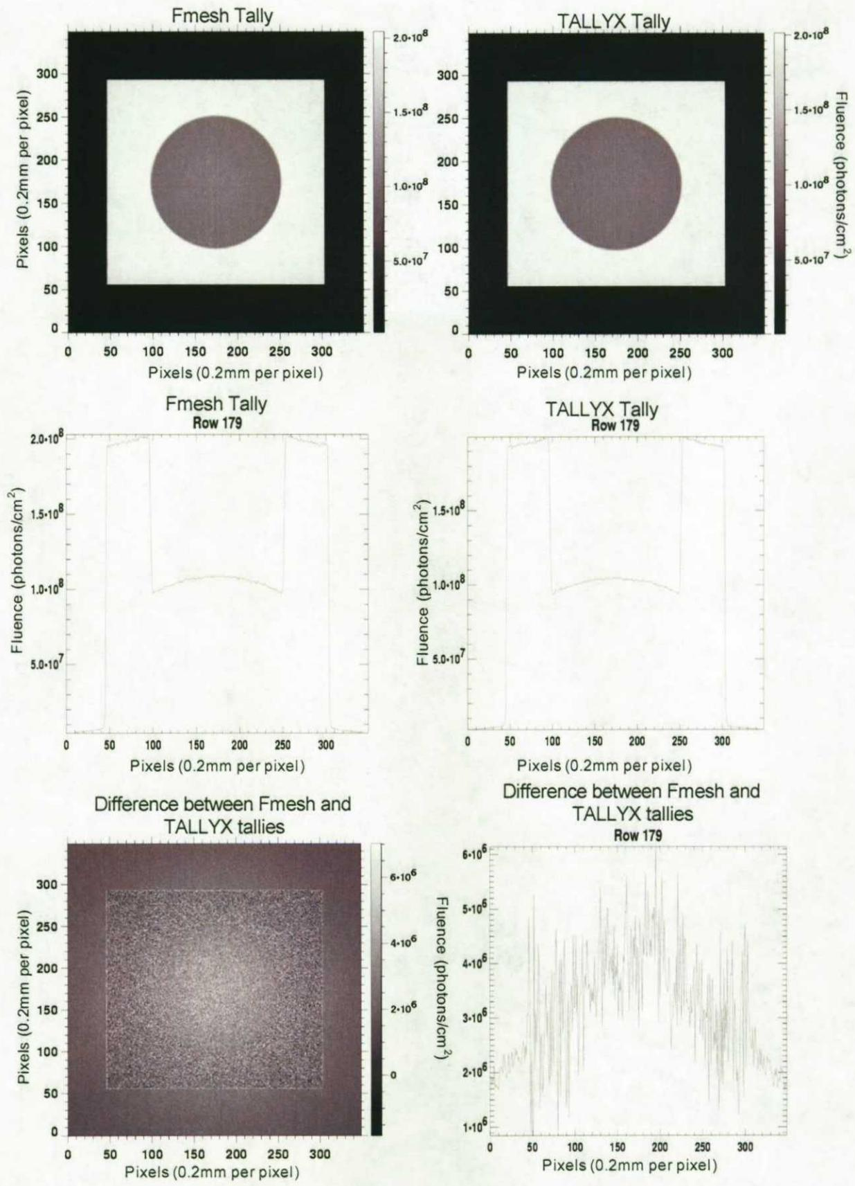
Figure 4 - Transmission images for the cylindrical target using the fmesh and TALLYX tallies.
