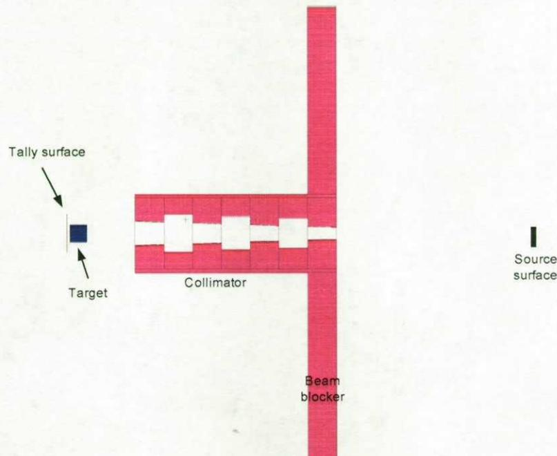
Figure 3- MCNP input geometries for the tagged cell simulated x-ray radiographs.
