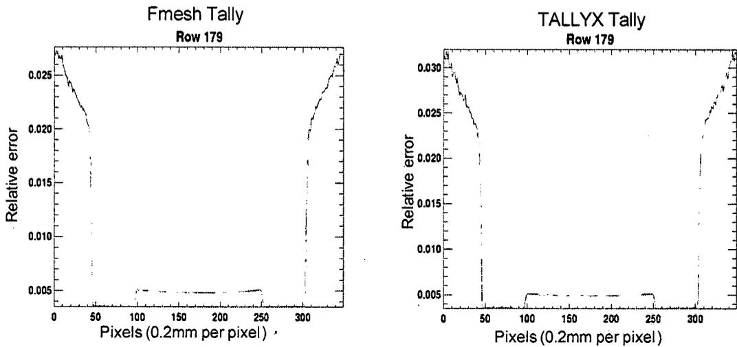
Figure 8- Line outs of the relative error of the fmesh and TALLYX tallies for the cylindrical target.
