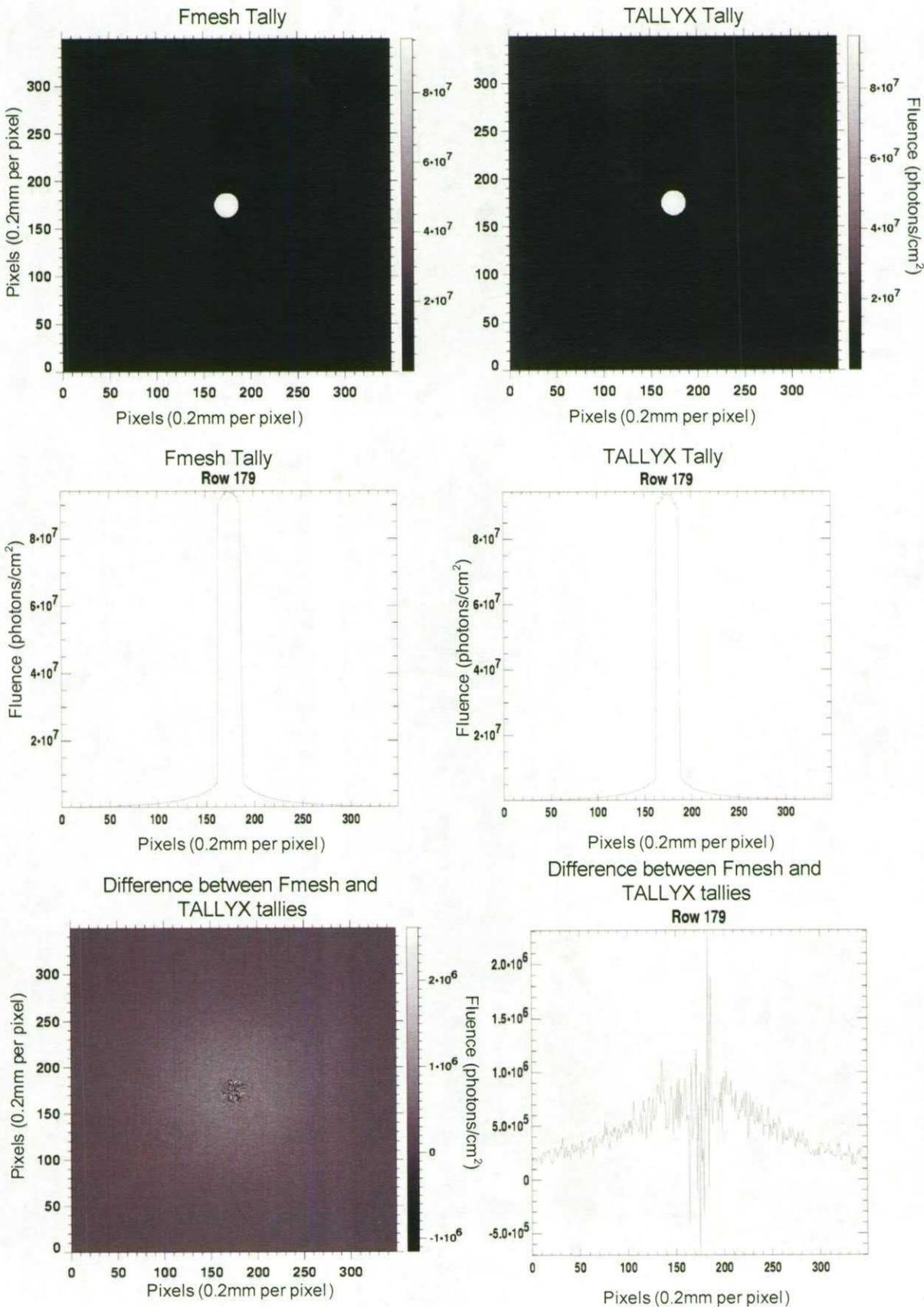
Figure 5 – Fmesh and TALLYX tagged cell tallies of cylinder 1.
