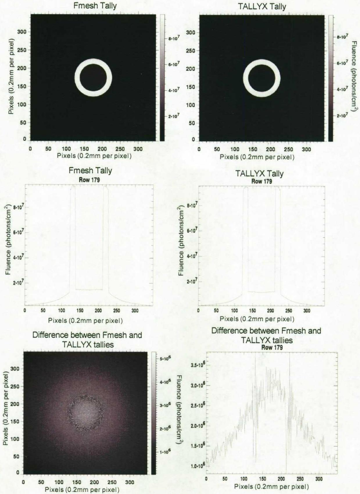
Figure 6- Fmesh and TALLYX tagged cell tallies of cylinder 4.
