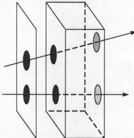
Figure 1- An illustration of two particles crossing the TALLYX surface tally pixel on the left and the fmesh volume tally voxel on the right.
