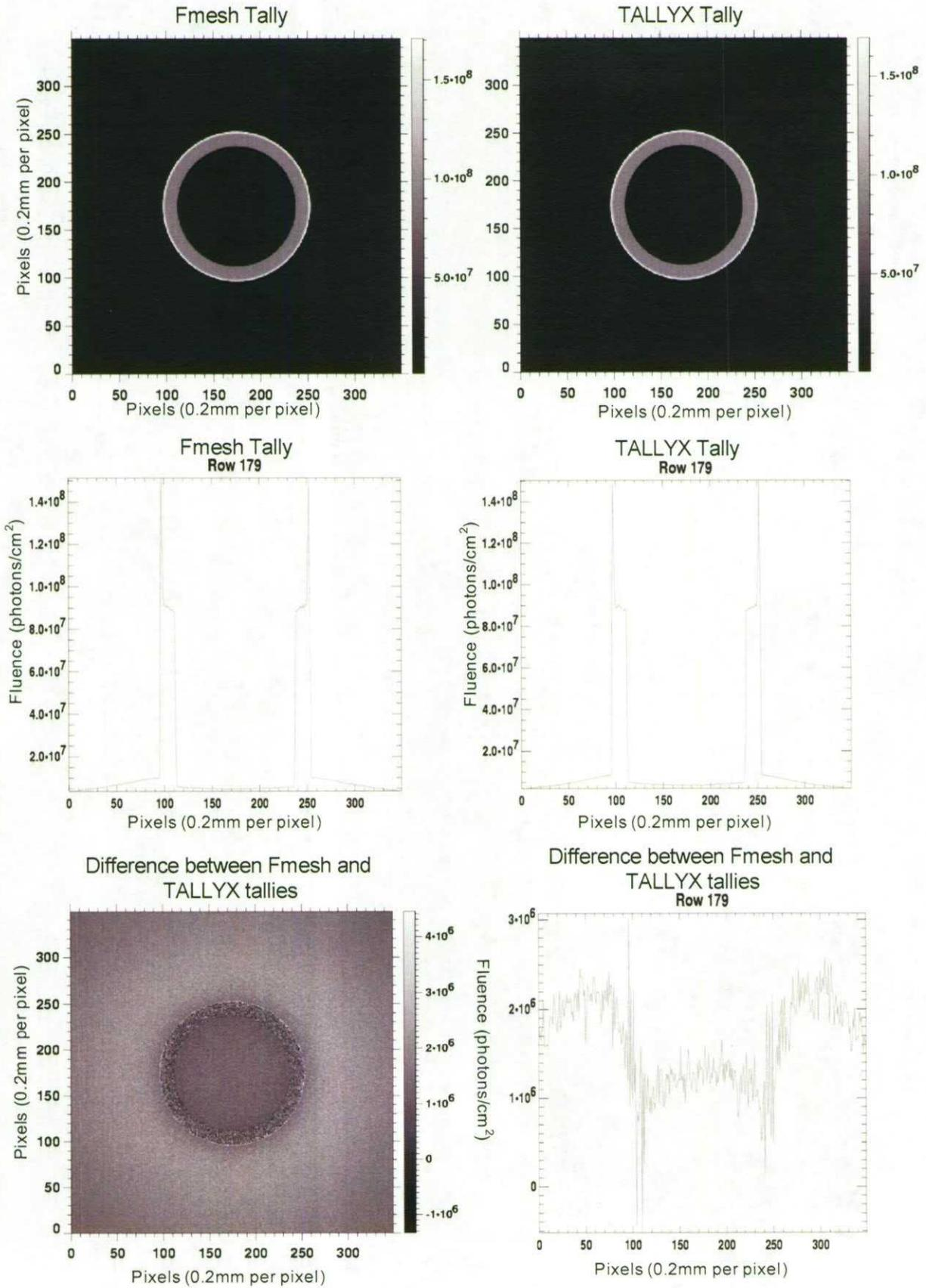
Figure 7- Fmesh and TALLYX tagged cell tallies of the outer cylinder (cylinder 6).
