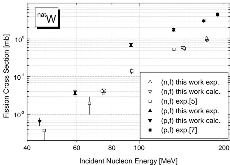
FIG. 4. The (n,f) and (p,f) cross-sections of  $^{nat}W$  versus incident nucleon energy.
