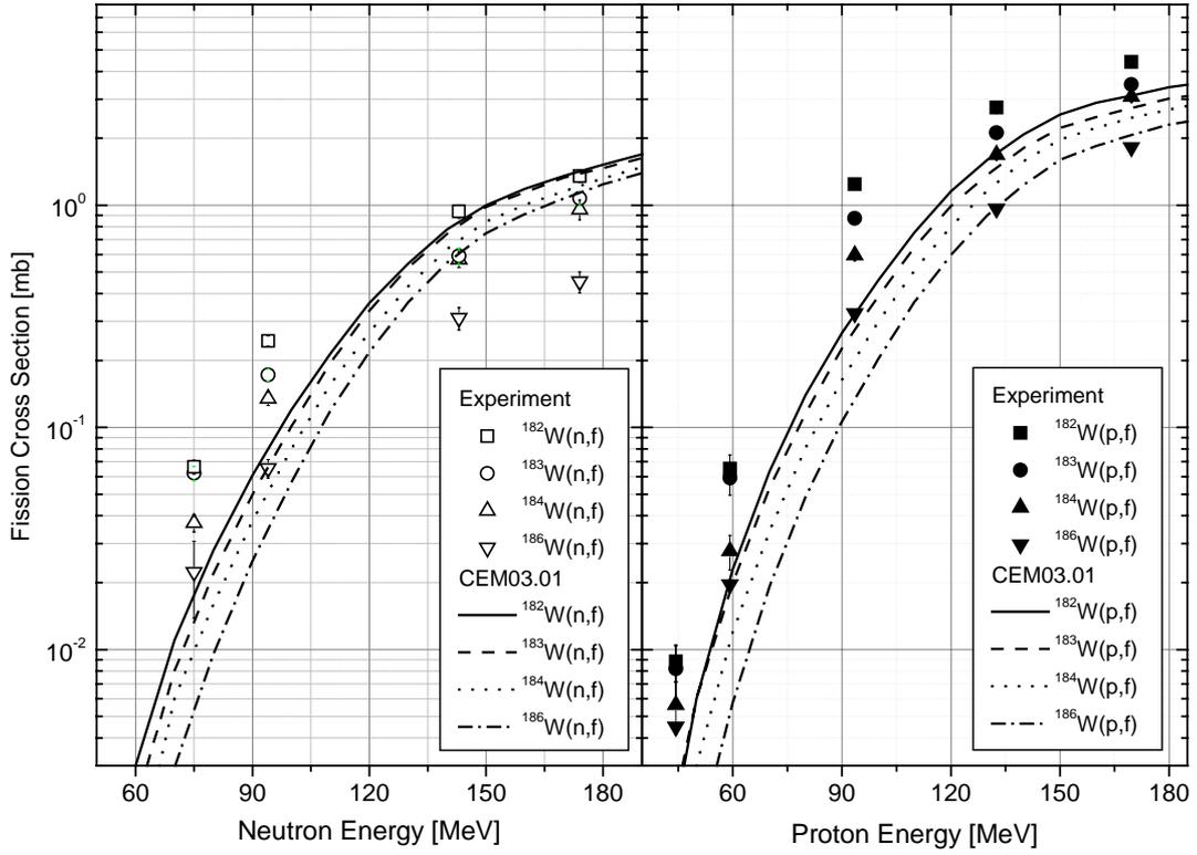
FIG. 1. The (n,f) and (p,f) cross-sections of  $^{182}\text{W}$ ,  $^{183}\text{W}$ ,  $^{184}\text{W}$ , and  $^{186}\text{W}$  versus incident nucleon energy. Symbols are experimental results of the present work, and curves are results of calculations by the CEM03.01 event generator [16].
