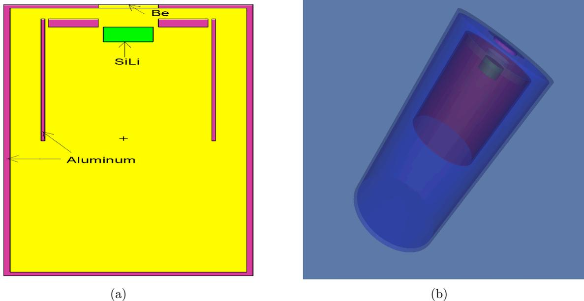
**Figure 1:** MCNP plot of SiLi detector
