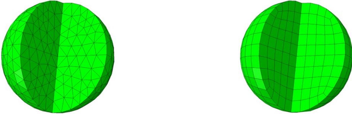
Figure 1. Simple Godiva sphere meshed with tetrahedrons (left) and hexahedrons (right) using seed values of 1.75 cm.
