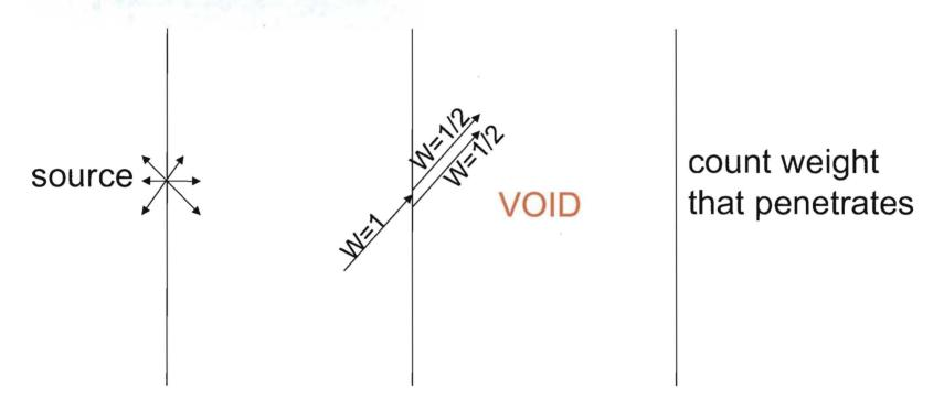
If both particles always do the same thing then no new information is gained from the split. Might as well save the computer time and not follow two particles doing exactly the same thing.
