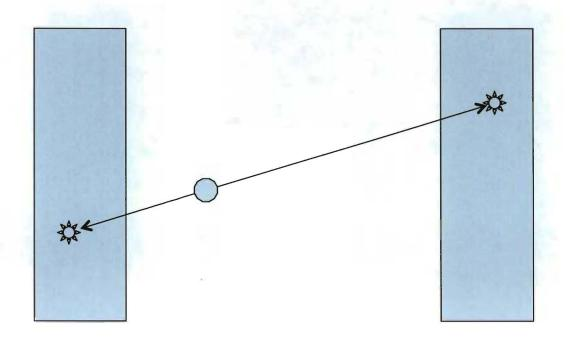
Two 0.511 MeV photons from pair annihilation event absorbed in a pulse height detector must contribute 1 hit in the 1.022 MeV bin and not two hits in the 0.511 Mev bin.
