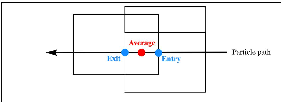
Figure: 3 - 1. Illustration of the three critical points for the overlap models.
