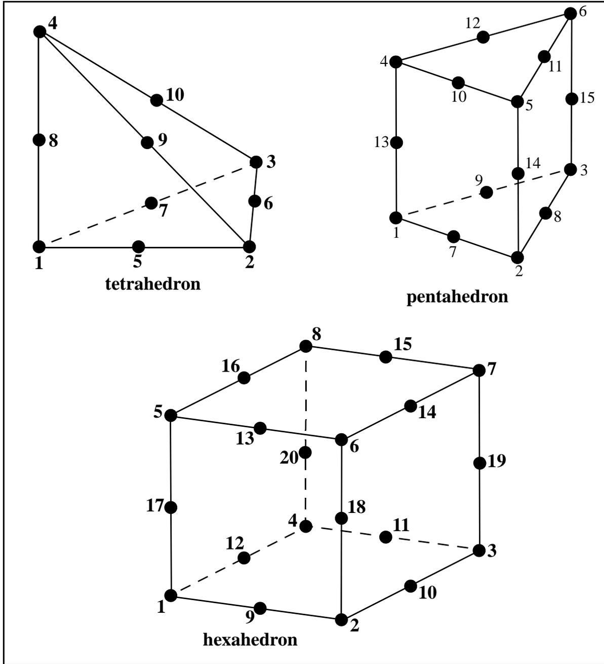
Figure: 2 - 1. Finite element types. For first order elements, ignore the midpoint nodes.
