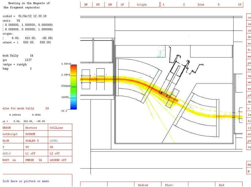
Primary ion beam as it collides with the beam dump
