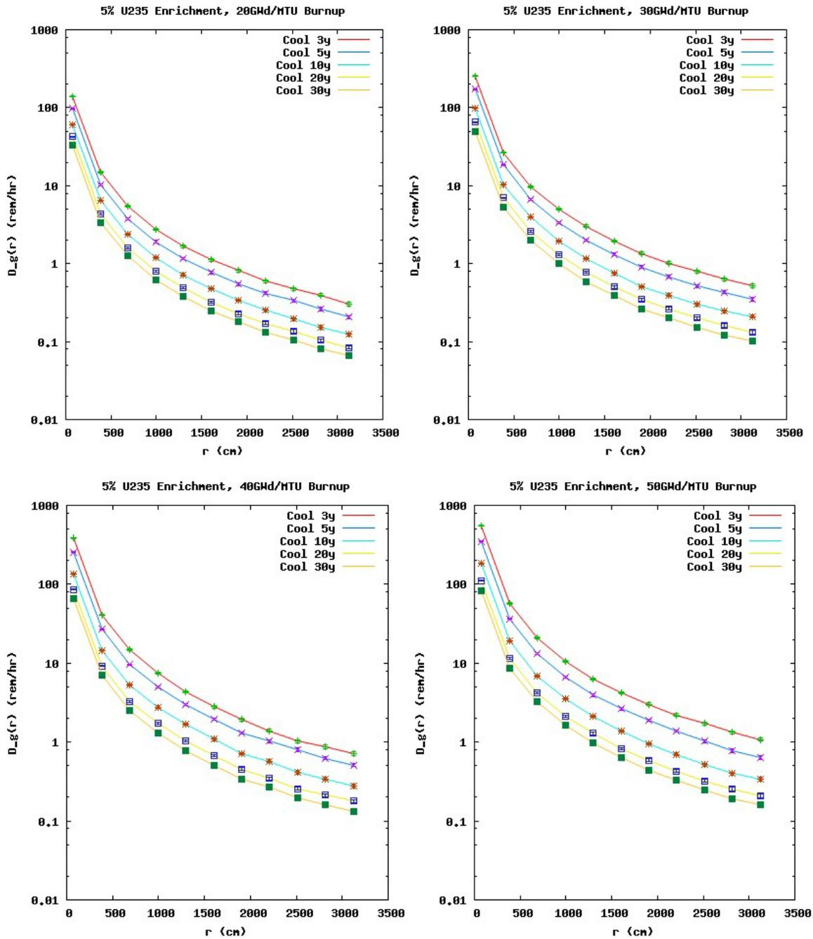
Figure 6. Photon dose rate as a function of distance for 5%  $^{235}\text{U}$  enrichment; 20, 30, 40, and 50 GWd/MTU burnup; and 3, 5, 10, 20, and 30 year cooling following irradiation.
