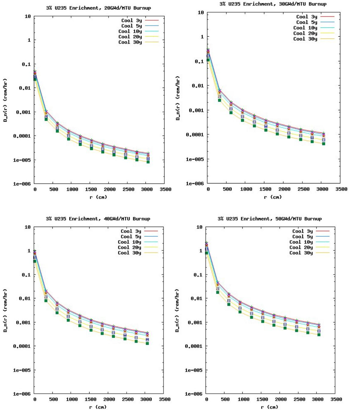
Figure 8. Neutron dose rate as a function of distance for 3%  $^{235}\text{U}$  enrichment; 20, 30, 40, and 50 GWd/MTU burnup; and 3, 5, 10, 20, and 30 year cooling following irradiation.
