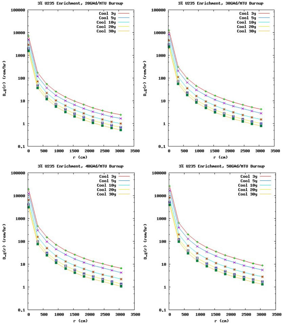
Figure 10. Photon dose rate as a function of distance for 3%  $^{235}\text{U}$  enrichment; 20, 30, 40, and 50 GWd/MTU burnup; and 3, 5, 10, 20, and 30 year cooling following irradiation.
