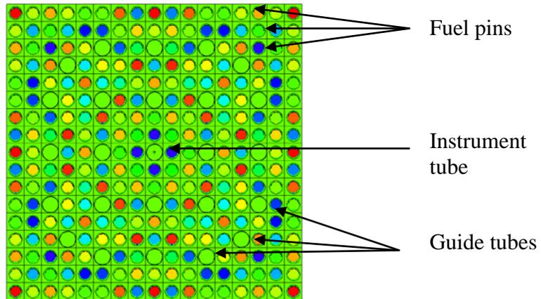
Figure 1. MCNP6 midplane fuel assembly geometry plot.
