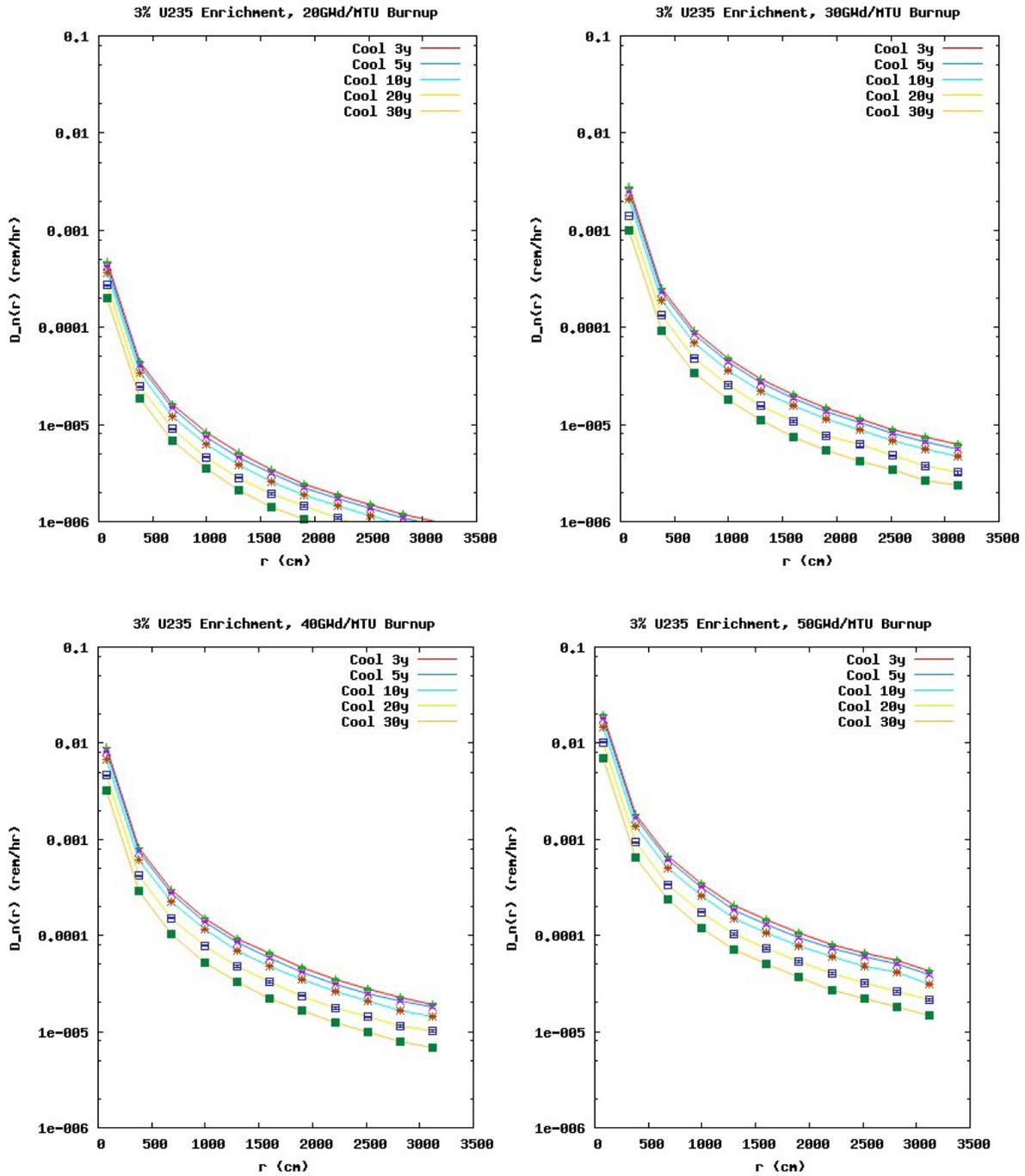
Figure 3. Neutron dose rate as a function of distance for 3%  $^{235}\text{U}$  enrichment; 20, 30, 40, and 50 GWd/MTU burnup; and 3, 5, 10, 20, and 30 year cooling following irradiation.
