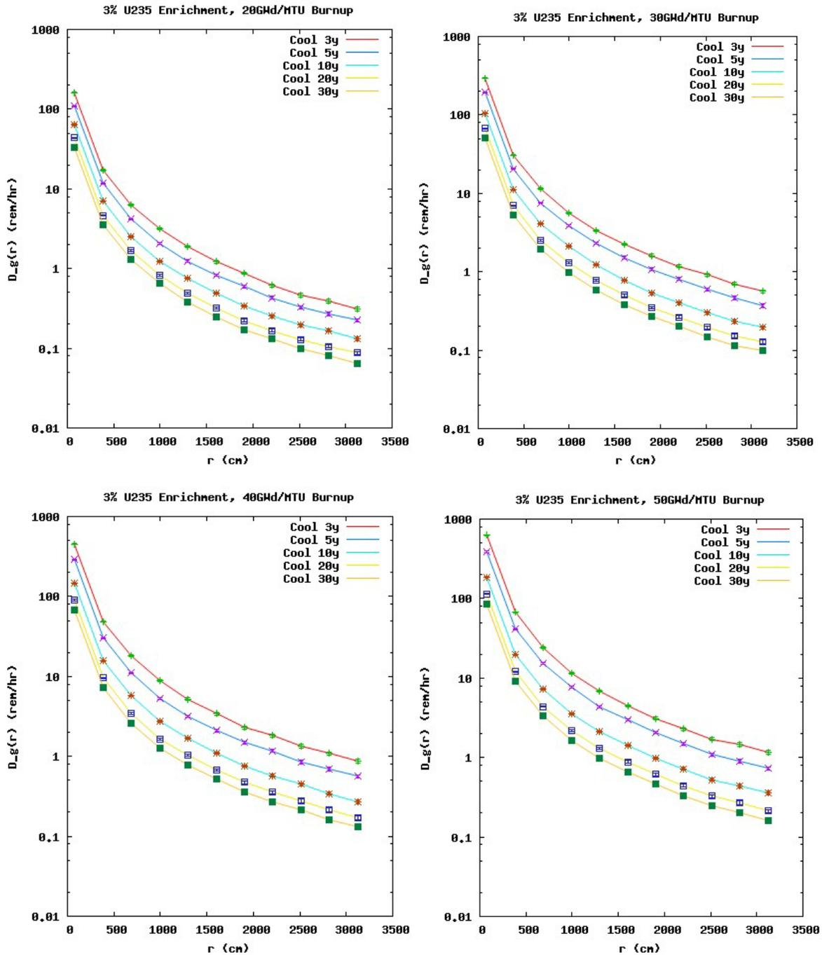
Figure 5. Photon dose rate as a function of distance for 3%  $^{235}\text{U}$  enrichment; 20, 30, 40, and 50 GWd/MTU burnup; and 3, 5, 10, 20, and 30 year cooling following irradiation.
