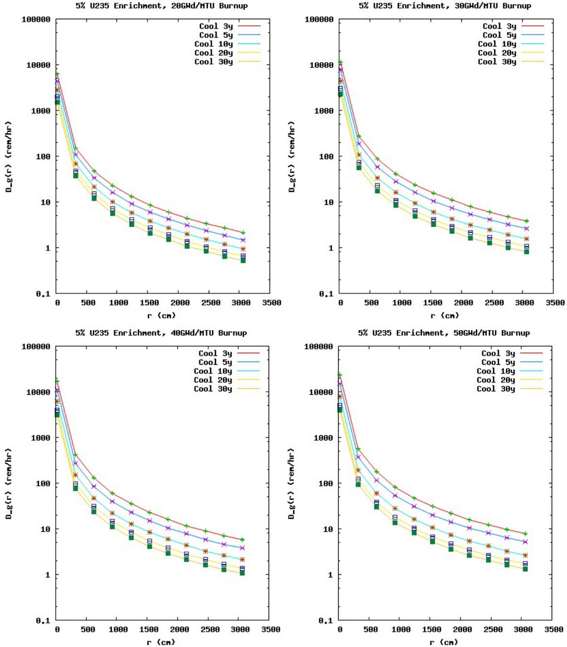
Figure 11. Photon dose rate as a function of distance for 5%  $^{235}\text{U}$  enrichment; 20, 30, 40, and 50 GWd/MTU burnup; and 3, 5, 10, 20, and 30 year cooling following irradiation.
