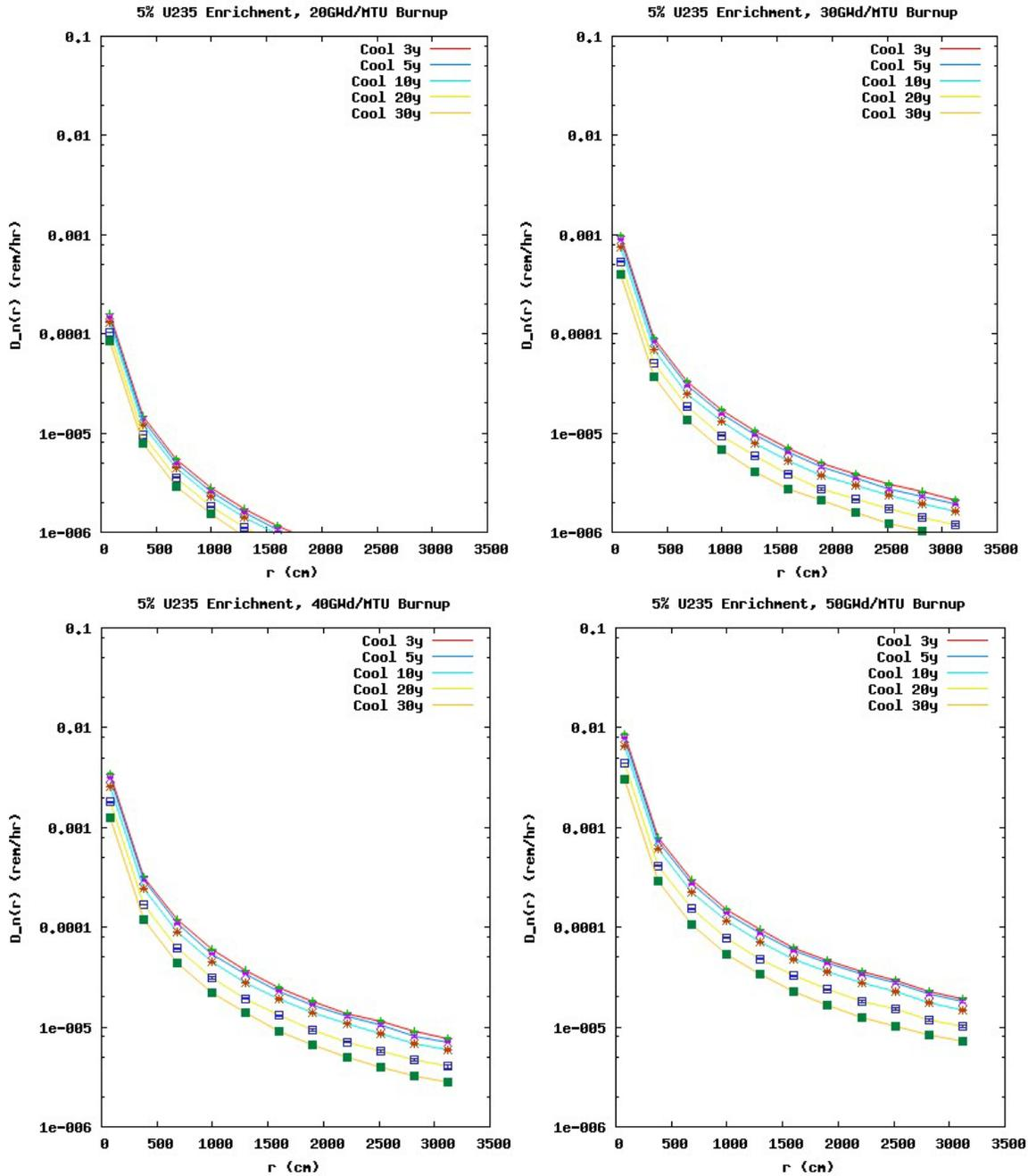
Figure 4. Neutron dose rate as a function of distance for 5%  $^{235}\text{U}$  enrichment; 20, 30, 40, and 50 GWd/MTU burnup; and 3, 5, 10, 20, and 30 year cooling following irradiation.
