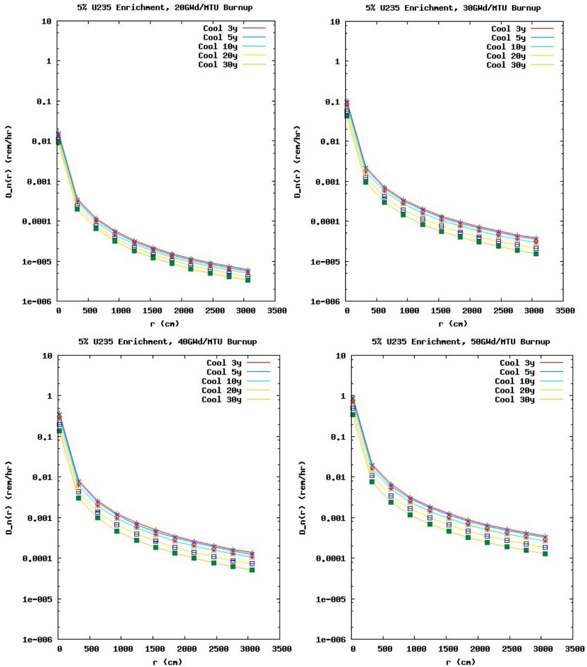
Figure 9. Neutron dose rate as a function of distance for 5%  $^{235}\text{U}$  enrichment; 20, 30, 40, and 50 GWd/MTU burnup; and 3, 5, 10, 20, and 30 year cooling following irradiation.
