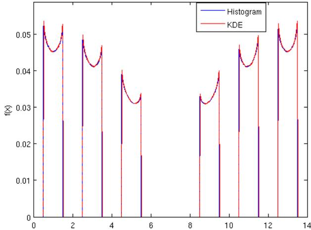
Fig. 5. Comparison of fission reaction rate profiles obtained from histogram and KDE collision tallies for the continuous-energy problem.
