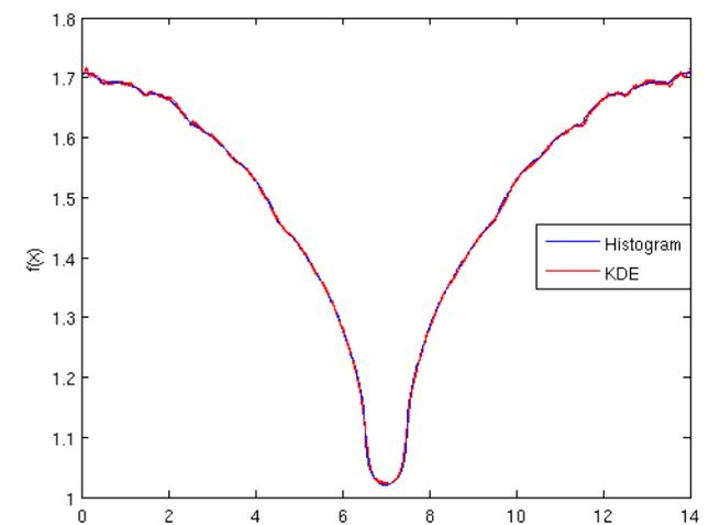
Fig. 4. Comparison of flux profiles obtained from histogram and KDE collision tallies for the continuous-energy problem.
