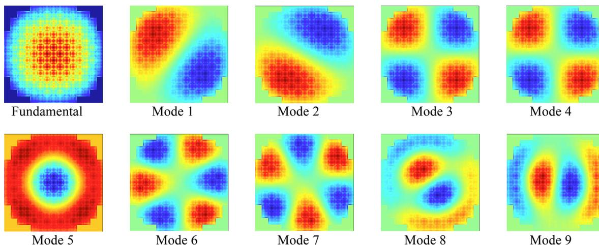
Figure 4. Fundamental and higher eigenmodes for 2D PWR model obtained from a fission matrix using a 60x60x1 spatial mesh.
