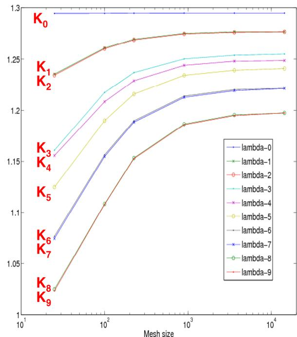
**Figure 9. Convergence of the first 10 eigenvalues for whole-core 2D PWR model as  $N$  is increased ( $N$  = spatial mesh cells for fission matrix tallies).**
