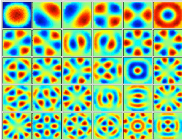
Figure 5. First 30 forward flux modes (top) of 2D PWR and relative uncertainties (bottom), Group 1 (0.625 eV – 20 MeV).
