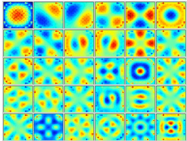
Figure 6. First 30 forward flux modes (top) of 2D PWR, and relative uncertainties (bottom), Group 2 (0 - 0.625 eV).
