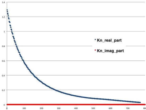
**Figure 7. Real and Imaginary parts of the 772 eigenvalues for the 2D PWR problem, using a 30x30 spatial mesh for fission matrix tallies.**
