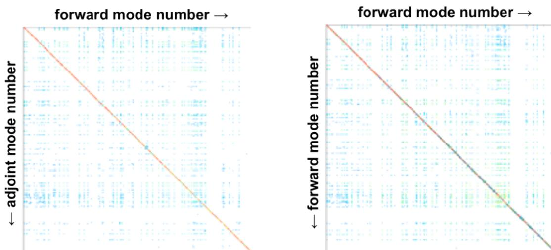
Figure 10. Biorthogonality of forward and adjoint fission source modes (left), and orthogonality of forward modes (right). Plotted points are inner products of modes. (scales: red - near 1.0, blue  $\leq 0.1$ )
