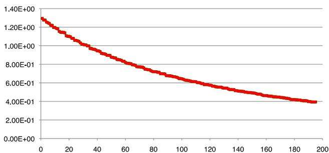
Figure 3. First 192 eigenvalues for 2D PWR problem, using a 120x120 spatial mesh for fission matrix tallies.
