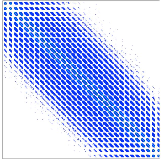
Figure 2. Fission matrix structure for 2D PWR
