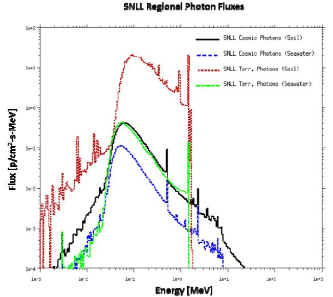
**Fig.3.** The four sources of photon surface spectra at or near Sandia National Laboratory – Livermore, CA: Cosmically induced over soil (black), cosmically induced over seawater (blue), terrestrially produced from soil (red), and terrestrially produced from seawater (green).
