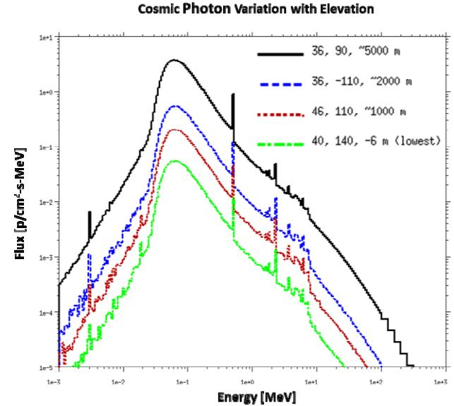
**Fig. 5.** Cosmic photon differential spectra for the locations specified in Fig. 4.
