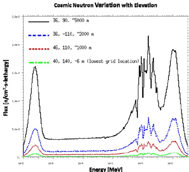
**Fig. 4.** Neutron lethargy spectra for several locations that vary in elevation, Tibetan region of China (black,  $36^{\circ}\text{N}$   $90^{\circ}\text{E}$ , elevation 16,476 feet), northeast of Flagstaff, AZ (blue,  $36^{\circ}\text{N}$   $110^{\circ}\text{W}$ , elevation 6,551 feet), western Mongolia (red,  $46^{\circ}\text{N}$   $110^{\circ}\text{E}$ , elevation 3,275 ft), and Hachirogata, Japan (green,  $40^{\circ}\text{N}$   $110^{\circ}\text{E}$ , elevation -20 ft).
