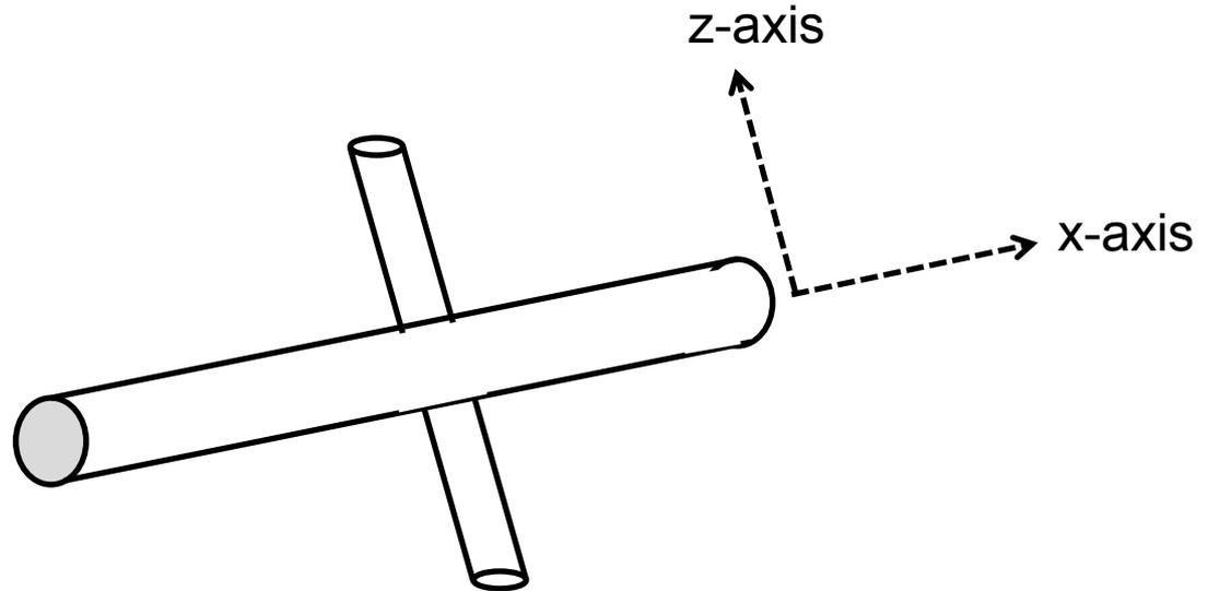
Void pipe through center of larger pipe ( $R=0.5$  cm). Length large enough to pass through larger pipe.
