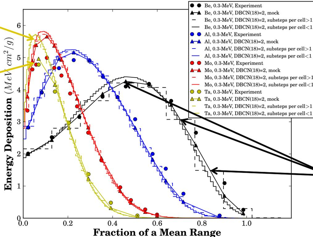
Profile is slightly sensitive to substeps per cell < 1
