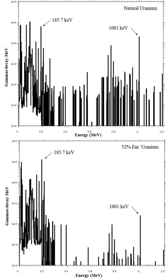
**Fig. 3** – Delayed gamma spectrum of natural (top) and 52% enriched uranium (bottom).
