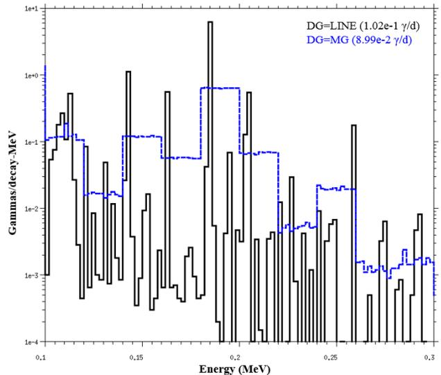
**Fig. 1** – Gamma emission spectrum from natural uranium for 0.1 to 0.3 MeV. Integral values are provided in parenthesis.
