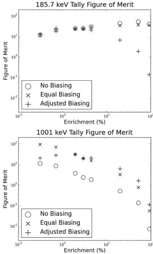
**Fig. 4** – Figure of merits for 185.7 keV (top) and 1001 keV (bottom) tallies using line-emission sampling
