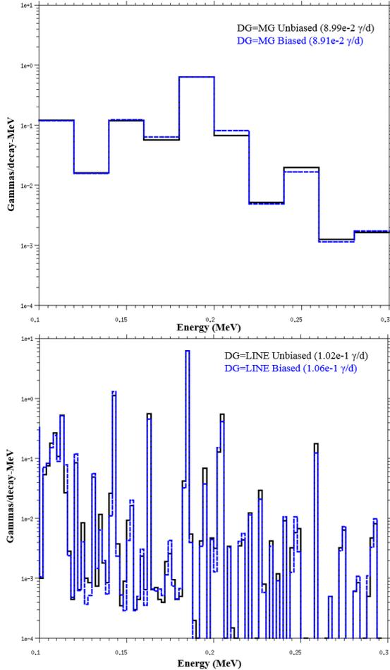
**Fig. 2** – Effects of biasing the 185.7 keV peak with multi-bin gamma sampling (top) and line-emission sampling (bottom). Integral values are provided in parenthesis.
