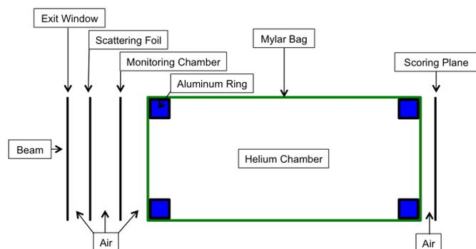
Figure 1: Schematic of experimental apparatus (not to scale).
