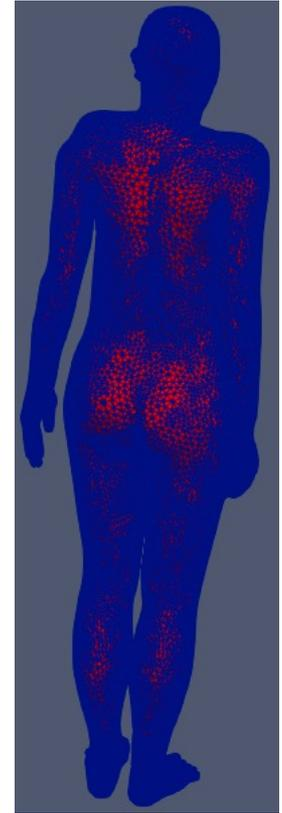
Element sets and instances are used to define the MCNP pseudo-cells.
