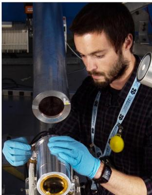
Keegan Kelly setting the 239Pu parallel plate avalanche counter for a Chi-Nu prompt fission neutron spectrum measurement.
