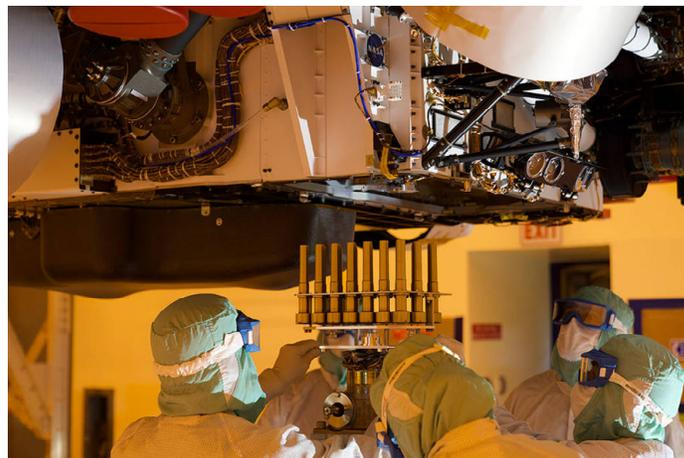
Sample tubes being installed in NASA's Perseverance Mars rover. The sample tubes are designed to be returned to Earth during later missions.
