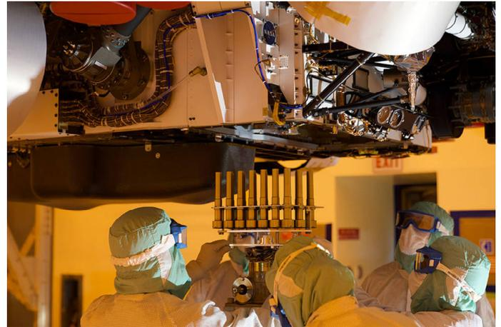
Sample tubes being installed in NASA’s Perseverance Mars rover. The sample tubes are designed to be returned to Earth during later missions. Credits: NASA/JPL-Caltech/KSC
