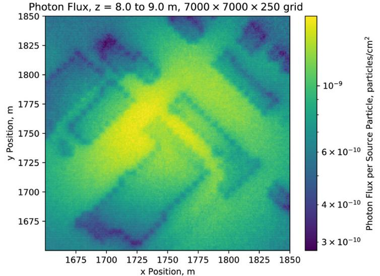
Plot of photon flux from a point source over a voxel mesh of Boston. Model courtesy of Tucker McClanahan.
