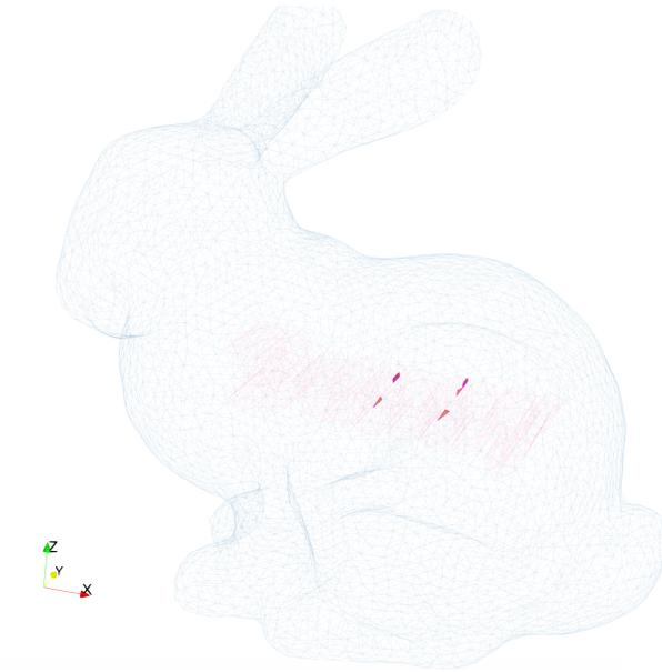
Figure 10: Extracted Poor-quality Elements with Model Wireframe
