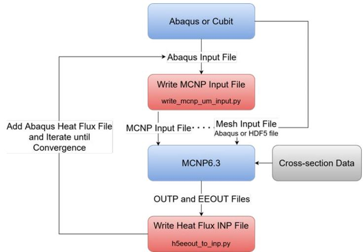
MCNP/Abaqus coupling calculations. This Python code is just a small portion of a bigger project at the Lab called MARM which, is a MCNP Abaqus-based reactor multiphysics software package being developed for microreactors.
