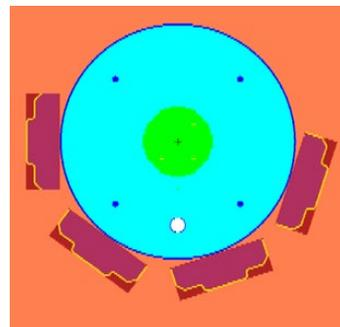
Top-down view of fuel-less assembly surrounded by four NoMAD detectors using MCPLOTTER. CREDIT: Tanner Heatherly
