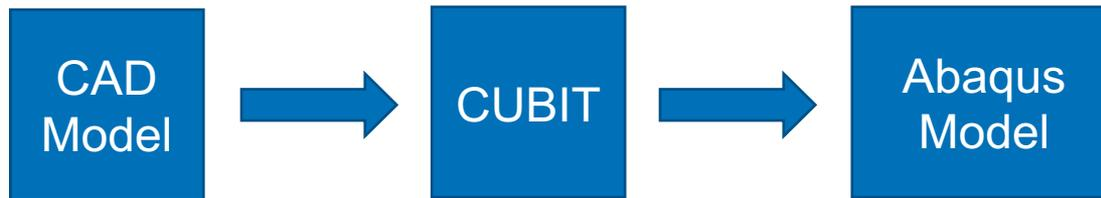
**MCNP cannot process Abaqus input files created by CUBIT. Python code was developed for file conversion.**
