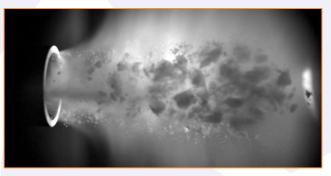
Cryogenic D-Ne shattered pellet exiting an injection system at 250 m/s (ORNL, 2021).
