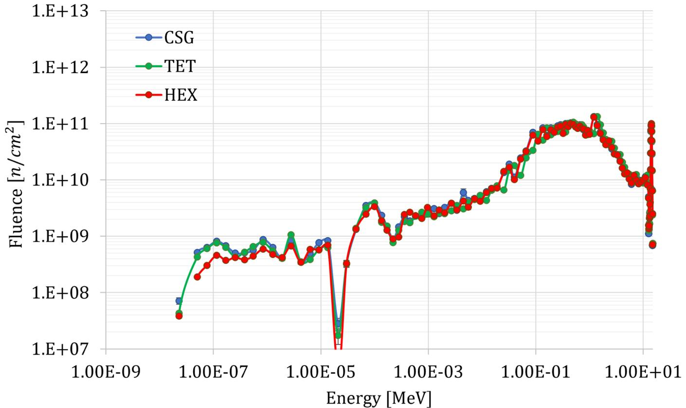
Figure 18. Total Neutron Fluence in Internal Drawer for CSG and UM Model Results from MCNP. Gamma fluence is not included because the experimental and calculation results were not reliable.
