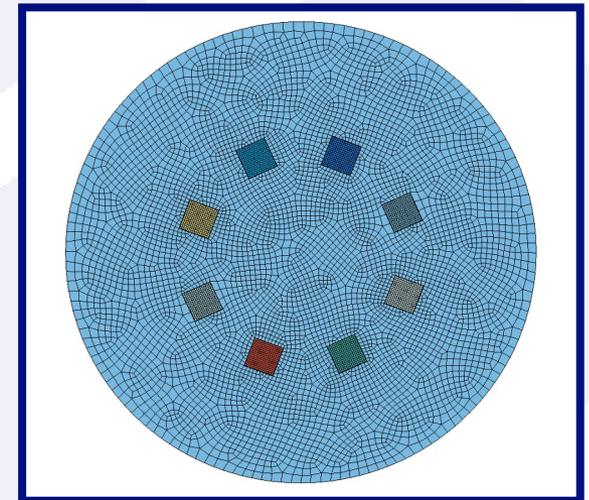
Figure 14. Zoomed View of TLDs Where Tally Calculations Occur (Foil are Below TLDs)
