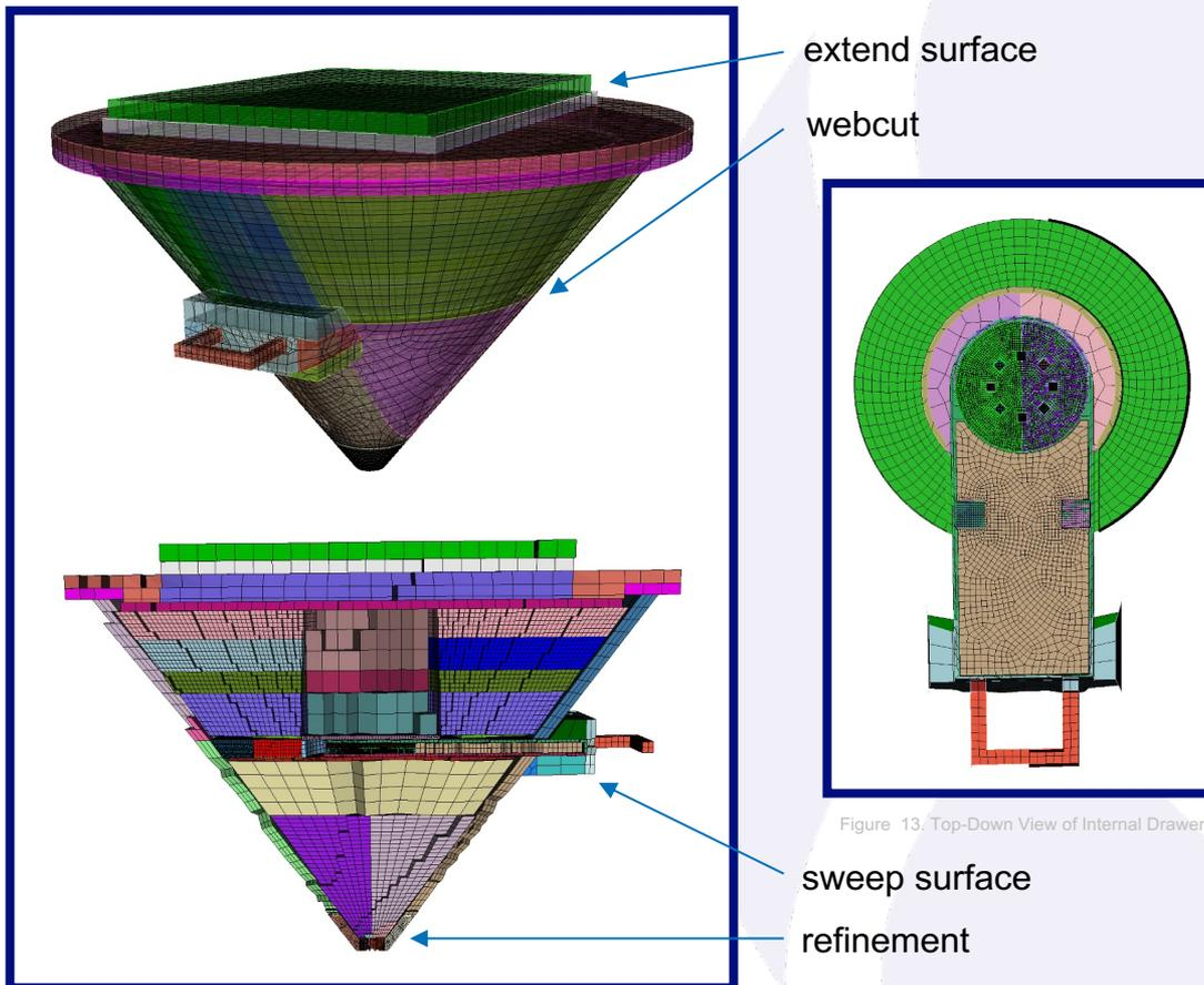
Figure 12. Isometric and Cross-Sectional View of Hex mesh model
