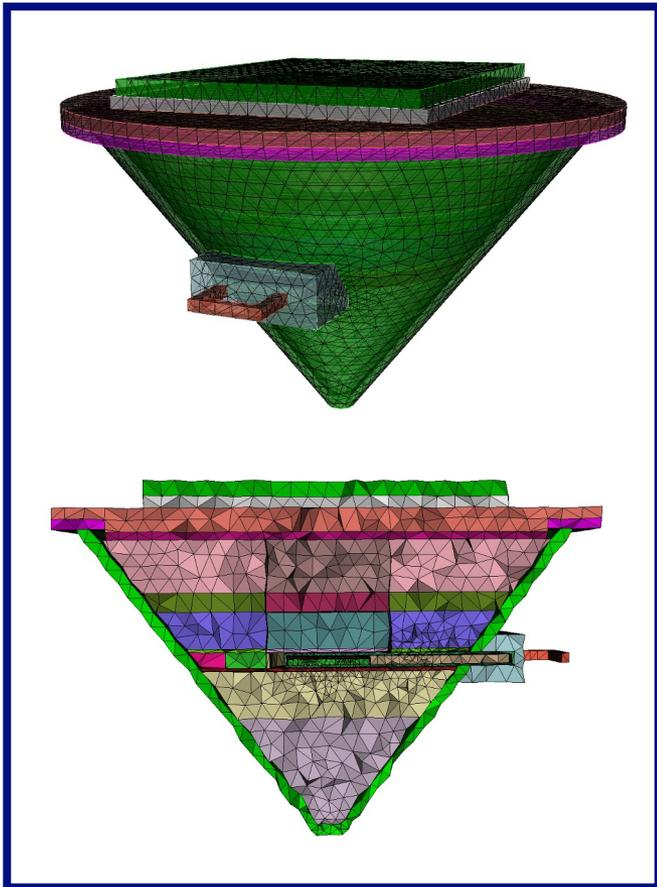
Figure 9. Isometric and Cross-Sectional View of Tet mesh model
