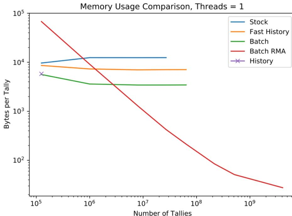
Batch RMA has high overhead that dissipates for large problems.
