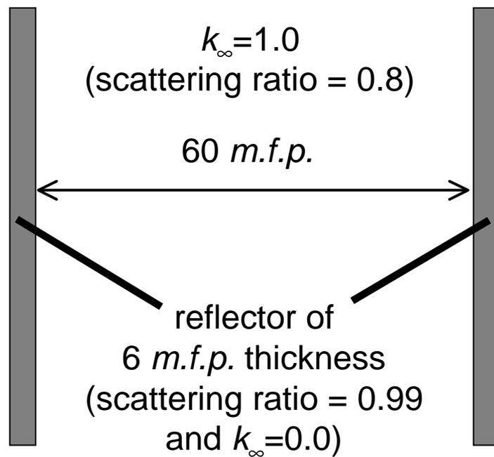
Figure 5: Energy-independent infinite slab reactor
