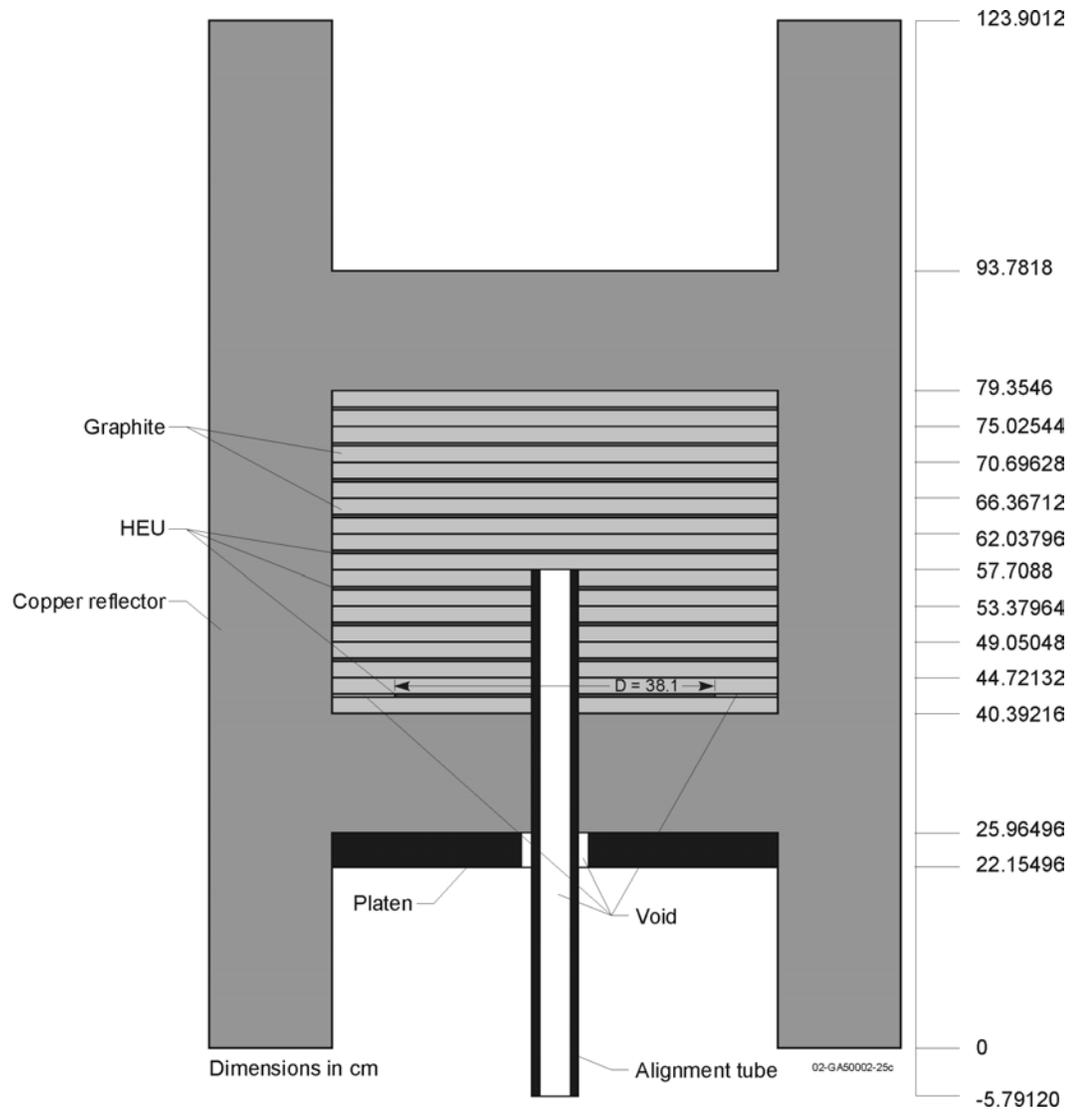
**Fig. 11.** Vertical Slice through the Benchmark Model of the Third Zeus Assembly.
