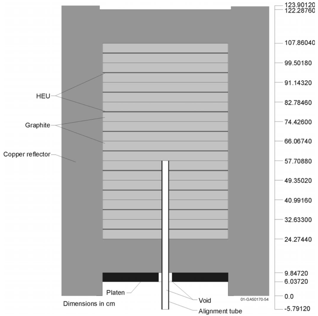
**Fig. 9.** Vertical Slice through the Benchmark Model of the First Zeus Assembly.
