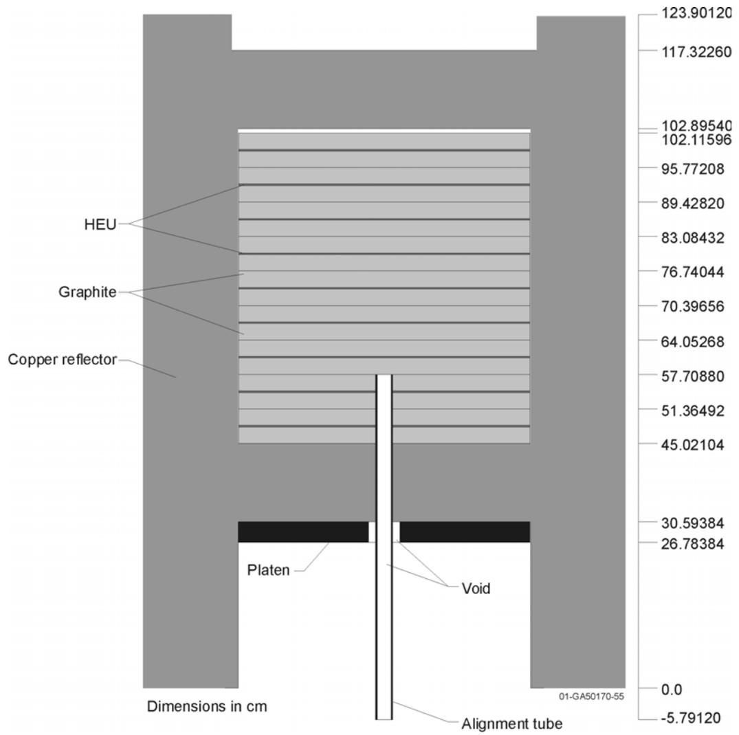
**Fig. 10.** Vertical Slice through the Benchmark Model of the Second Zeus Assembly.
