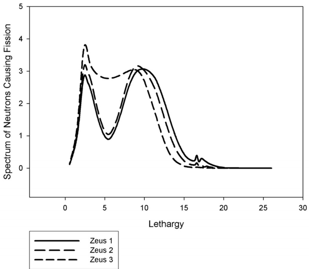
**Fig. 8.** Spectra of Neutrons Causing Fission in Zeus Fuel Platters.
