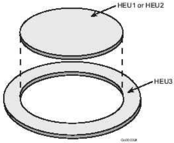
**Fig. 2.** Structure of Zeus Fuel Platters.
