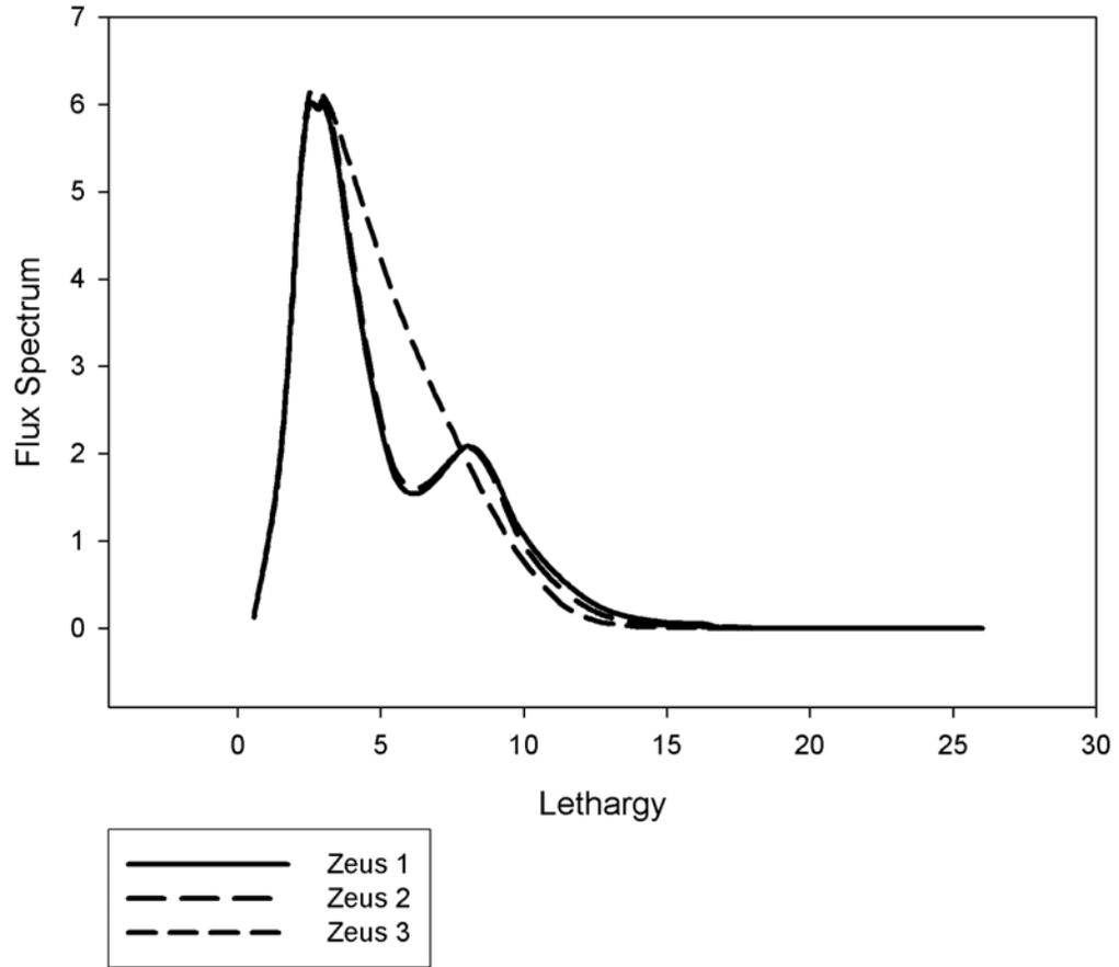
**Fig. 7.** Flux in Zeus Fuel Platters.
