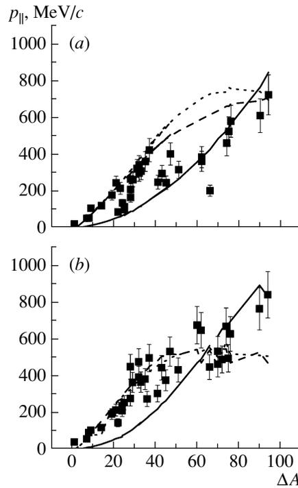
**Fig. 2.** Dependence of average longitudinal momentum on the number of emitted nucleons: (a) for deuteron-induced reactions, (b) for proton-induced reactions. Curves show calculations (solid) by LAQGSM03.01, (dashed) by LAQGSM03.S1, and (dotted) by LAQGSM03.G1.
