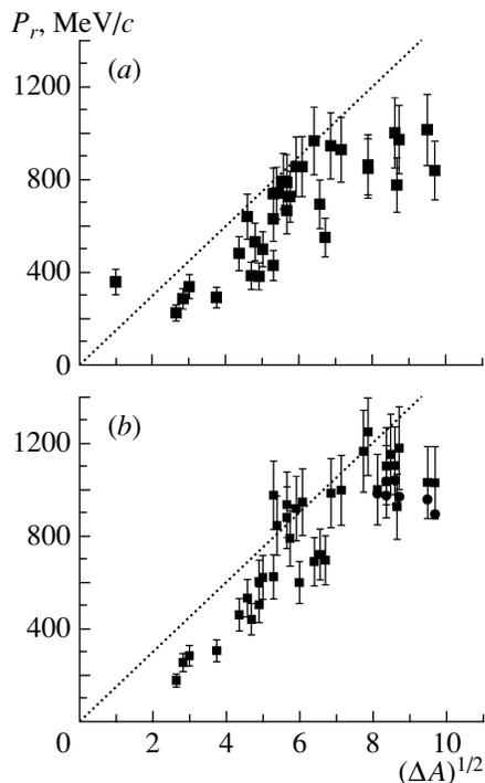
**Fig. 3.** The momentum of recoil nuclei as a function of observed mass loss: (a) for deuteron-induced reactions, (b) for proton-induced reactions. Dotted line is the systematics of Morrissey [1].
