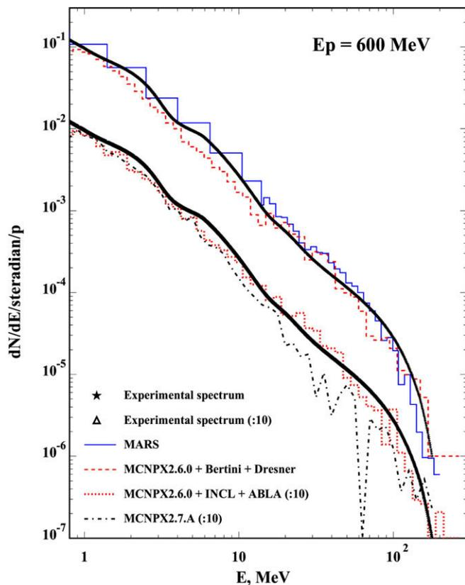
Fig. 7. Experimental neutron spectrum for 0.6 GeV initial proton energy and calculation by the MARS code and the MCNPX code.
