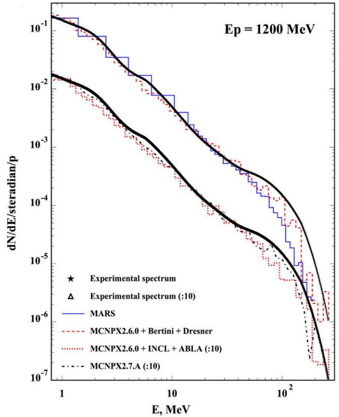
Fig. 4. Experimental neutron spectrum for 1.2 GeV initial proton energy and calculation by the MARS code and the MCNPX code.
