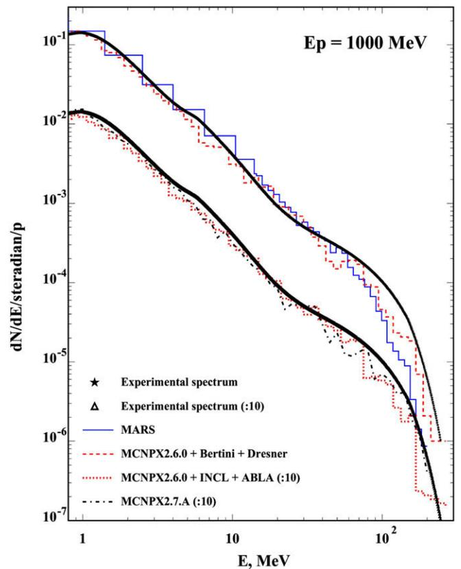
Fig. 5. Experimental neutron spectrum for 1.0 GeV initial proton energy and calculation by the MARS code and the MCNPX code.
