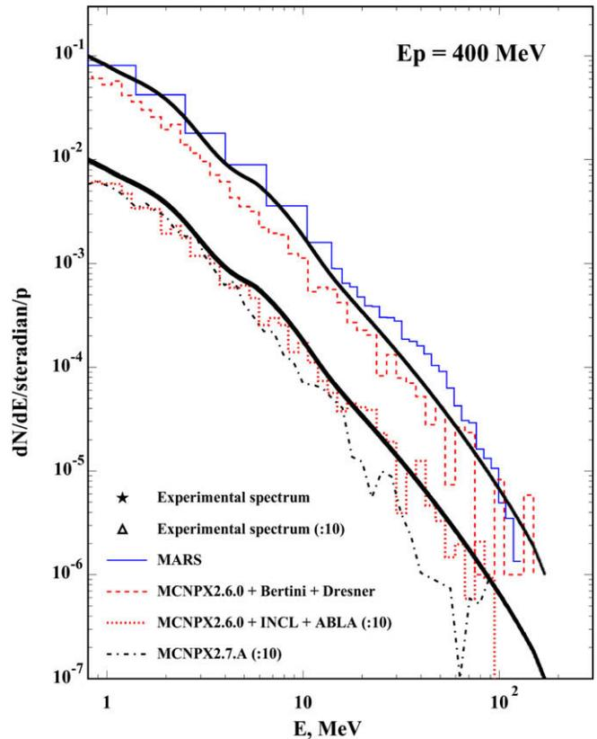
Fig. 8. Experimental neutron spectrum for 0.4 GeV initial proton and calculation by the MARS code and the MCNPX code.
