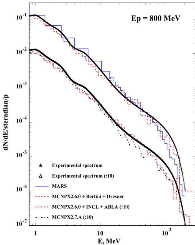
Fig. 6. Experimental neutron spectrum for 0.8 GeV initial proton energy and calculation by the MARS code and the MCNPX code.
