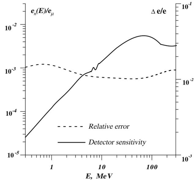
Fig. 2. Detector sensitivity to neutron; solid line corresponds to the left scale while dashed line, to the right one.
