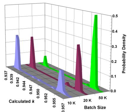
Fig. 1. Distribution of MCNP calculated *k* for various batch sizes.
