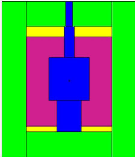
Big Ten is a stack of concentric cylinders. The inner and outer radii of the depleted uranium are 26.67 and 41.91 cm, respectively. The total length of the configuration is 96.52 cm.
