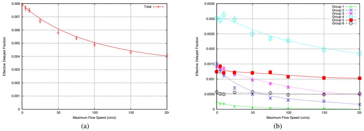
Figure 3: Changes in total (a) and individual components of (b)  $\beta_{\text{eff}}$  for various flow rates.
