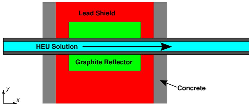
Figure 1: Geometry of the Flowing Uranyl Nitrate Solution Case.
