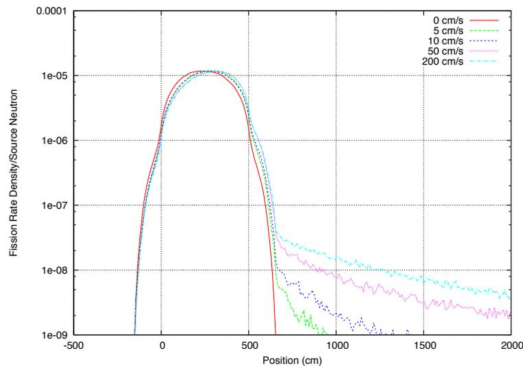
Figure 2: **Shift in fundamental mode for increasing flow rates.**
