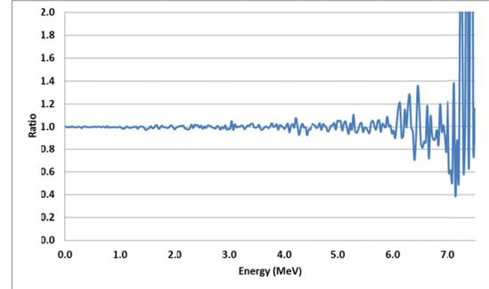
Figure 1. Ratios of F1 tally results between unbiased and energy biased delayed particles. The small fluctuations about 1.0 show proper convergence of the technique.
