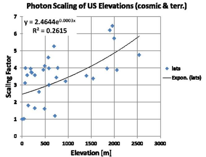
Fig. 3. Integral photon fluxes from terrestrial US grid-point locations, along with the corresponding exponential fit for terrestrially and cosmically produced photons.
