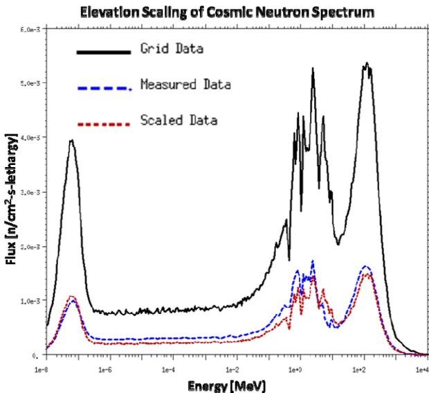
Fig. 2. Spectrum from background.dat at 38° N, 120° W, 1,695 m grid point (black) and scaled to SNLL location 37.7° N, 122.7° W, 196 m (red) where measured data was taken (blue). The scaling function value of 0.2779 was applied to scale from 1,695 m to 196 m.
