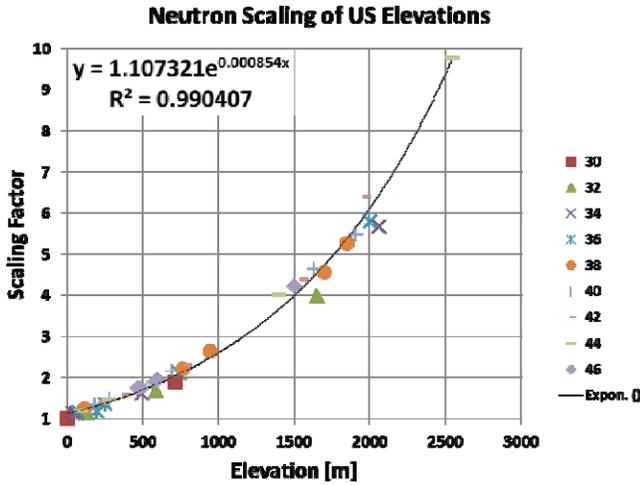
Fig. 1. Integral neutron fluxes from terrestrial US grid-point locations along with the corresponding exponential fit used to scale grid elevations to user's input. Scaling factors are demarked by latitude.
