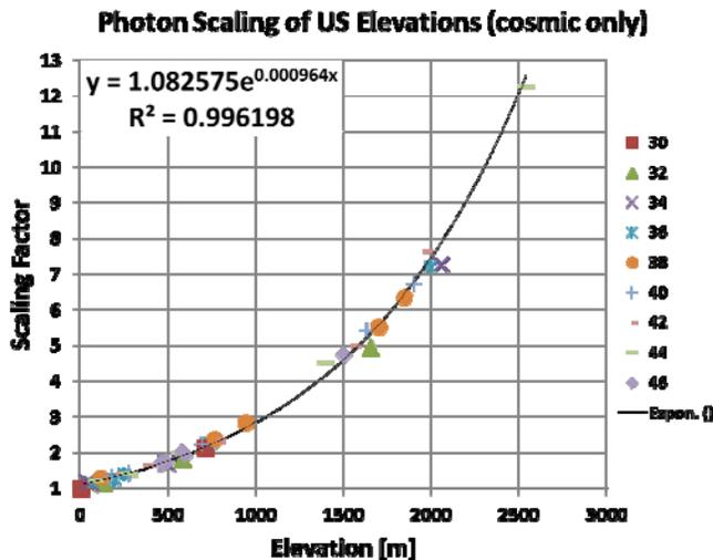
Fig. 4. Integral photon fluxes from terrestrial US grid-point locations along with the corresponding exponential fit for cosmically produced photons only.
