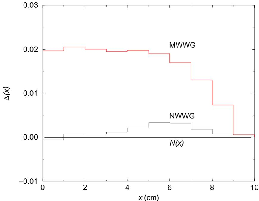
**Fig 1. Fractional difference between the estimated importance, Eq. (12), and the analytical importance, Eq. (4), for  $c = 0.1$  and  $\sigma = 0.2$  /cm. NWWG and MWWG refer to the new and existing MCNP weight window generators.**
