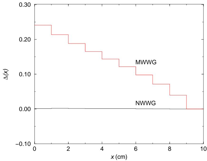
**Fig 2. Fractional difference between the estimated importance, Eq. (12), and the analytical importance, Eq. (4), for  $c = 0.9$  and  $\sigma = 0.2$  /cm. NWWG and MWWG refer to the new and existing MCNP weight window generators.**
